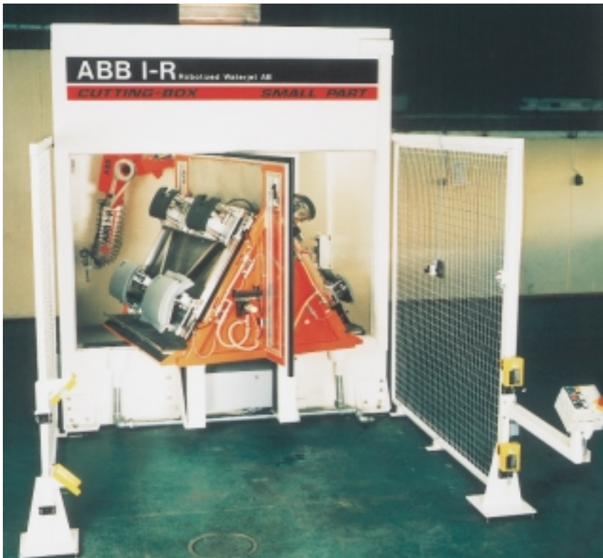
'Lean' concept for cutting small plastics parts based on the 'Cutting Box Small Part'. Full utilization is made of the limited space by inclining the rotary worktable.
