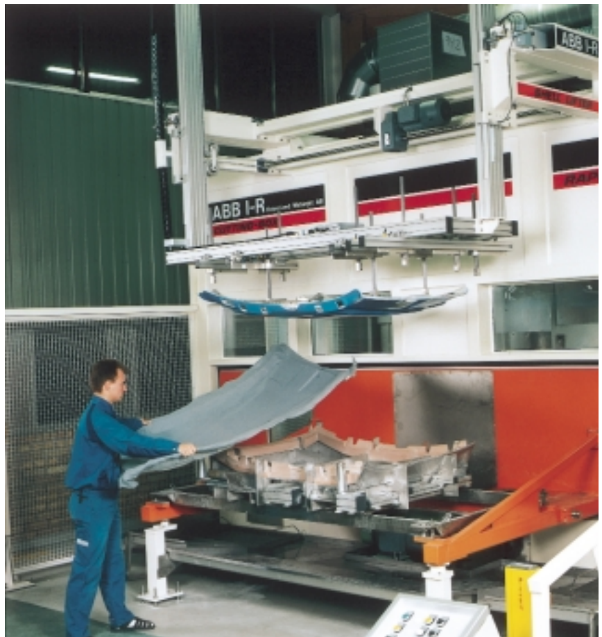
'Cutting Box Original', equipped with two type IRB 2400 robots and an automatic shell-lifter, used to cut car headliners
