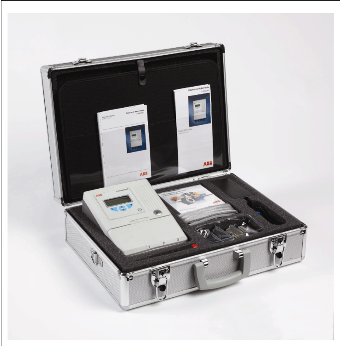
Fig. 2-4: C2C uses ABB's CalMaster2 in-situ verification system to ensure the continued accuracy of its installed AquaMaster flow meter
