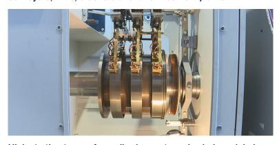
High starting torque from slip-ring motors also helps minimise mechanical stresses on the driven equipment, increasing the lifetime of the equipment and reducing maintenance needs.
