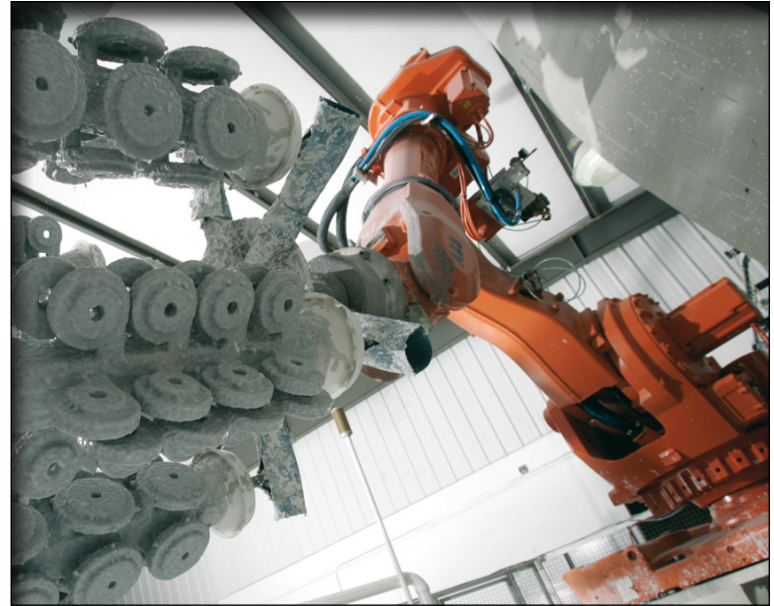
An ABB IRB 6600 robot is part of a complete shelling system for investment casting company Franklin Bronze and Alloy.
