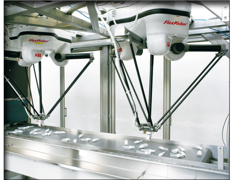
ABB FlexPicker robots pack tubes of pharmaceuticals in a compact cell built by Italy-based Industria Macchine Automatiche.
