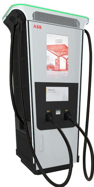
The Terra 360 CC model in UL configuration with CCS1 dual outlet cable connectors, shown with credit card reader, and a 27" advertising screen.
