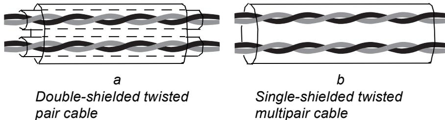
Run analogue and digital signals in separate cables.
