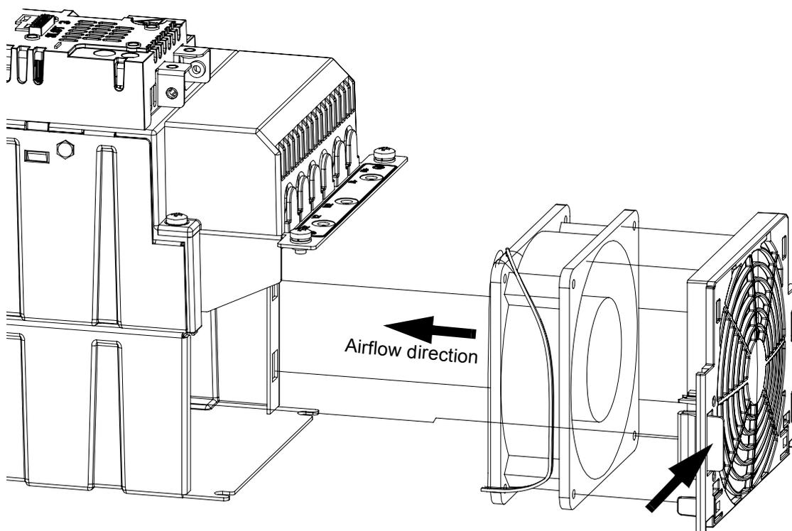
**Fan replacement (Frames C and D, ACSM1-04Cx-xxxx-x)**
