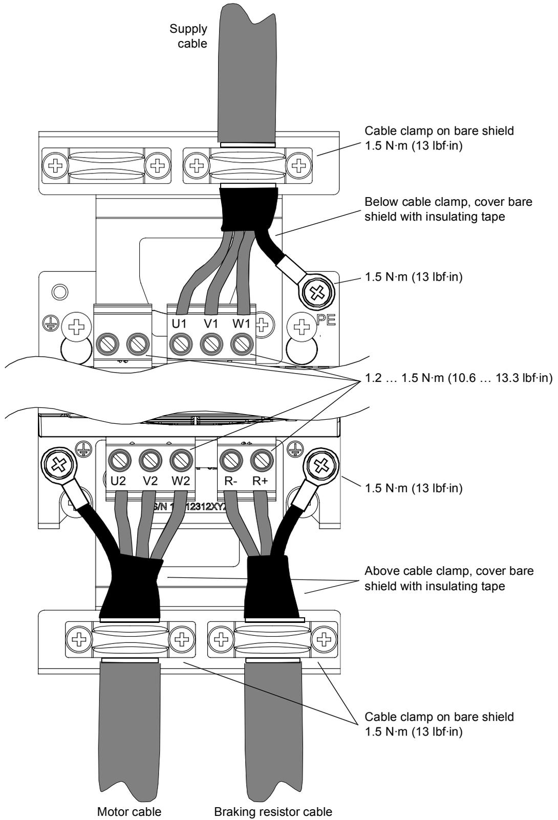
Power cable connection – frame sizes C and D (connector covers removed)
