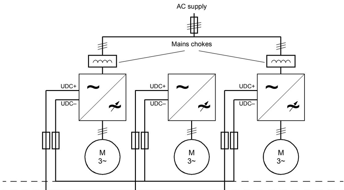
Each drive has an independent DC capacitor pre-charging circuit.
