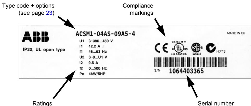
The first digit of the serial number refers to the manufacturing plant. The 2nd and 3rd digit indicate the year of manufacture, while the 4th and 5th digits indicate the week. Digits 6 to 10 are a running integer starting every week at 00001.
