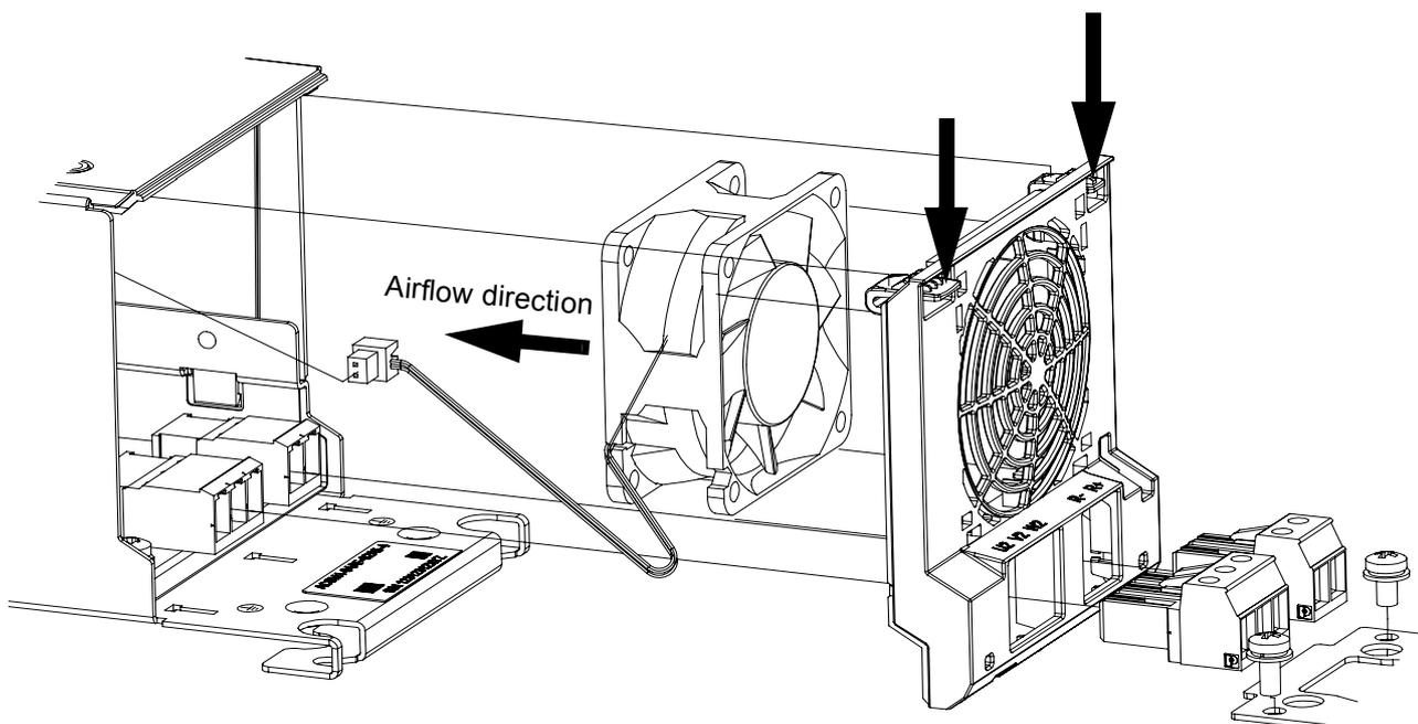
**Fan replacement (Frames C and D, ACSM1-04Ax-xxxx-x)**
