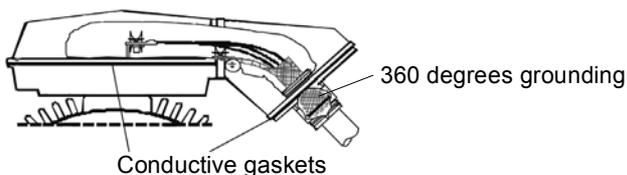
or ground the cable by twisting the shield so that the flattened shield is wider than 1/5 of its length.
