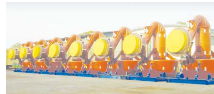
For semisubmersible drilling rigs ABB provides refurbishment, storage and exchange of rotation pods (Azipod® CZ thrusters).
