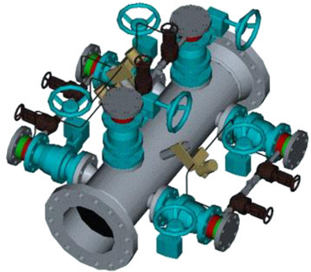
Fig. 8 Solid model of wedge meter with redundant transmitter capability
