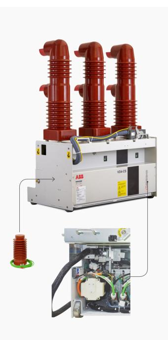
To support your business needs in reactive power compensation, ABB offers dedicated vacuum circuit breaker with servomotor actuation and controlled switching up to 38kV, 1250A, 31.5kA and up to 20,000 operations with extremely low probability of re-strike and transients minimization in capacitor bank switching. Additionally with VD4-CS1 real time power factor compensation and reactor switching are allowed.
