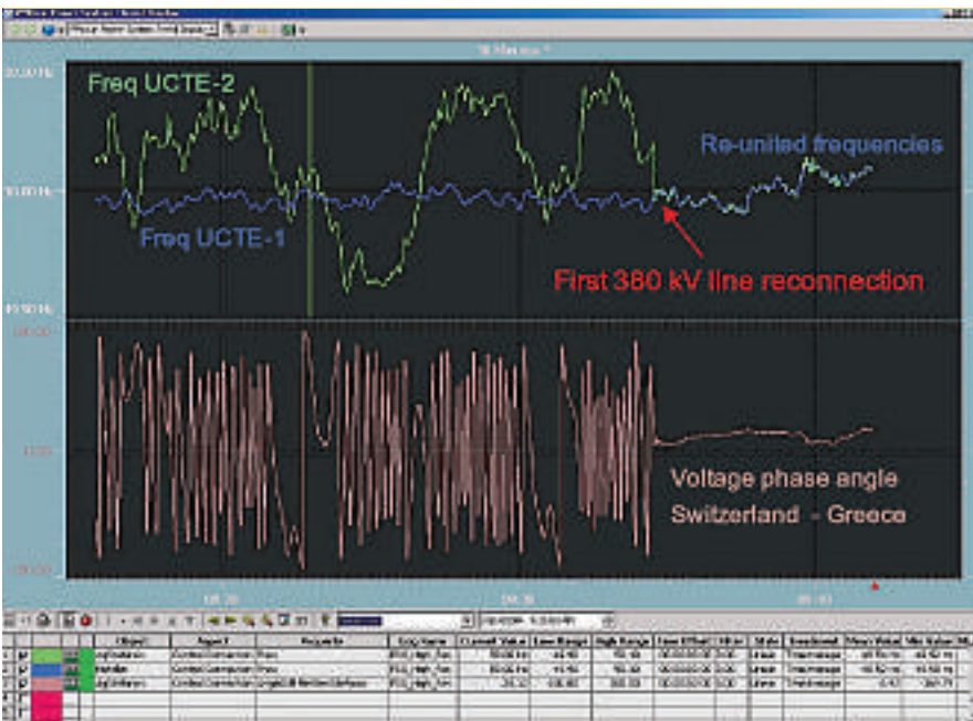
5 PSGuard on-line trend display: UCTE-1 and UCTE-2 voltage phase angle difference and frequencies during the historical resynchronization process recorded by PSGuard.
