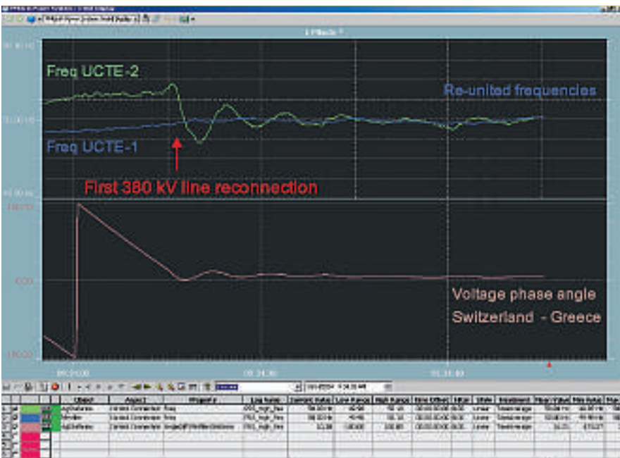
6 PSGuard on-line trend display: zoom functionality (1 minute) to exactly display the behavior of the power grid dynamics after the first 380 kV line reconnection (Arad – Sandorfalva).
