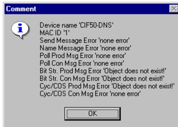
Figure 26: Information on a device in the automatic scan window
