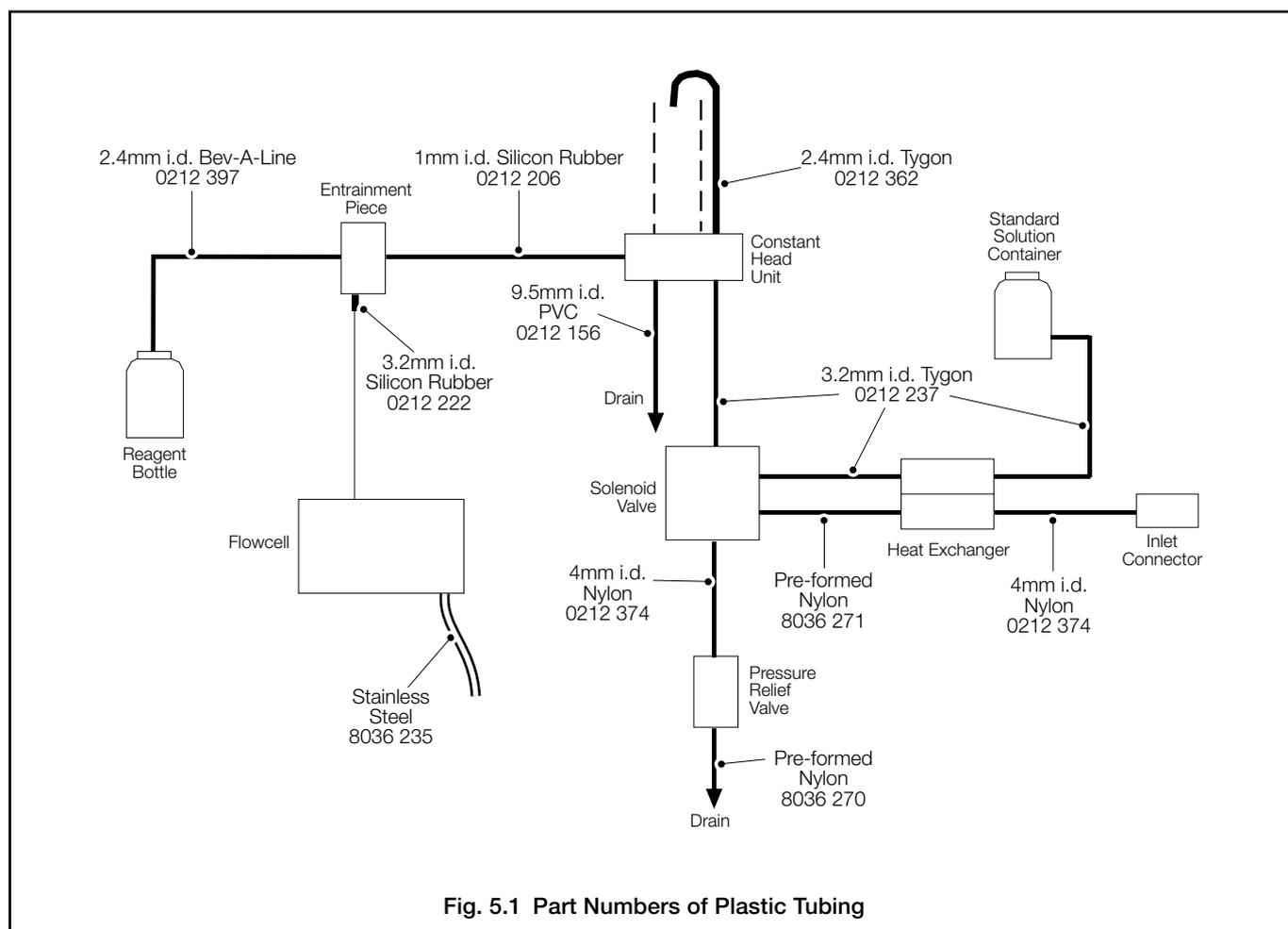
Fig. 5.1 Part Numbers of Plastic Tubing
