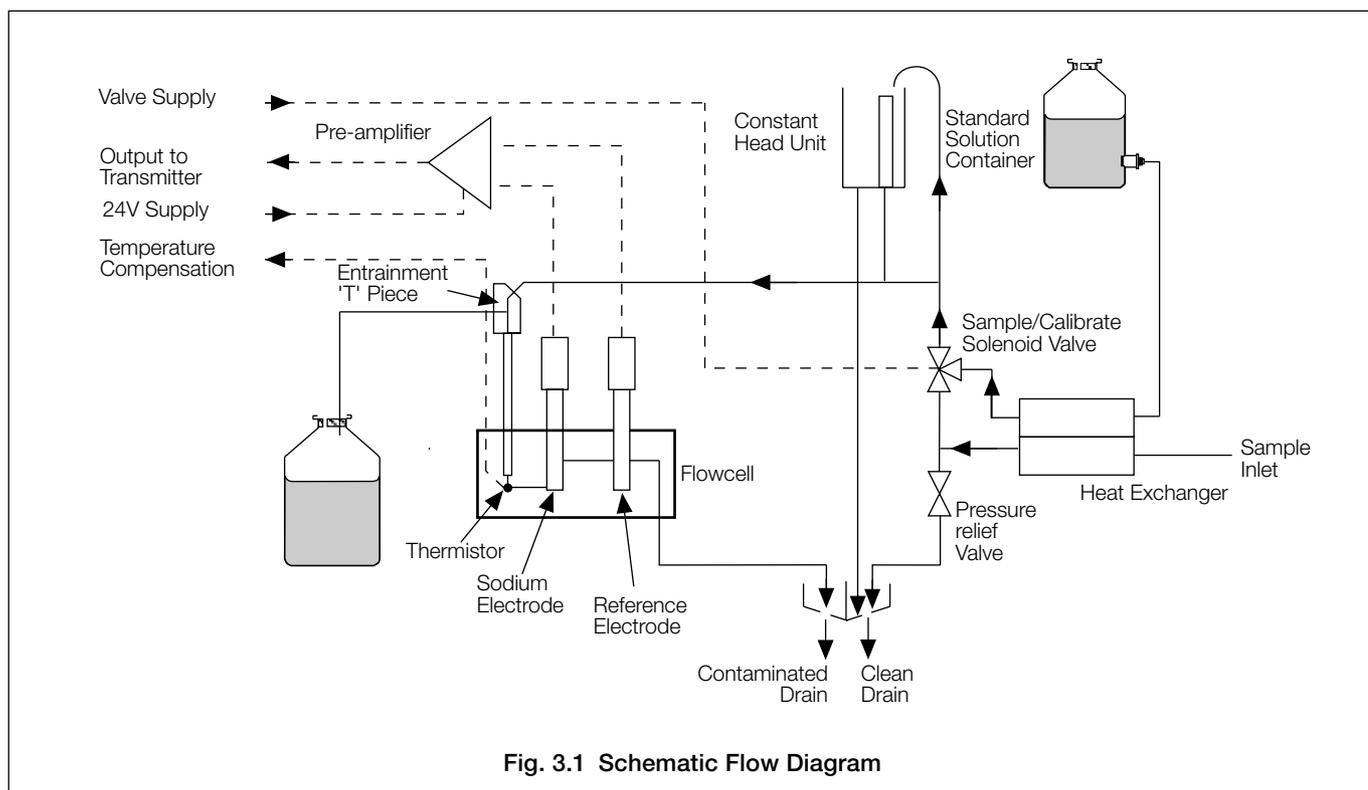
Fig. 3.1 Schematic Flow Diagram
