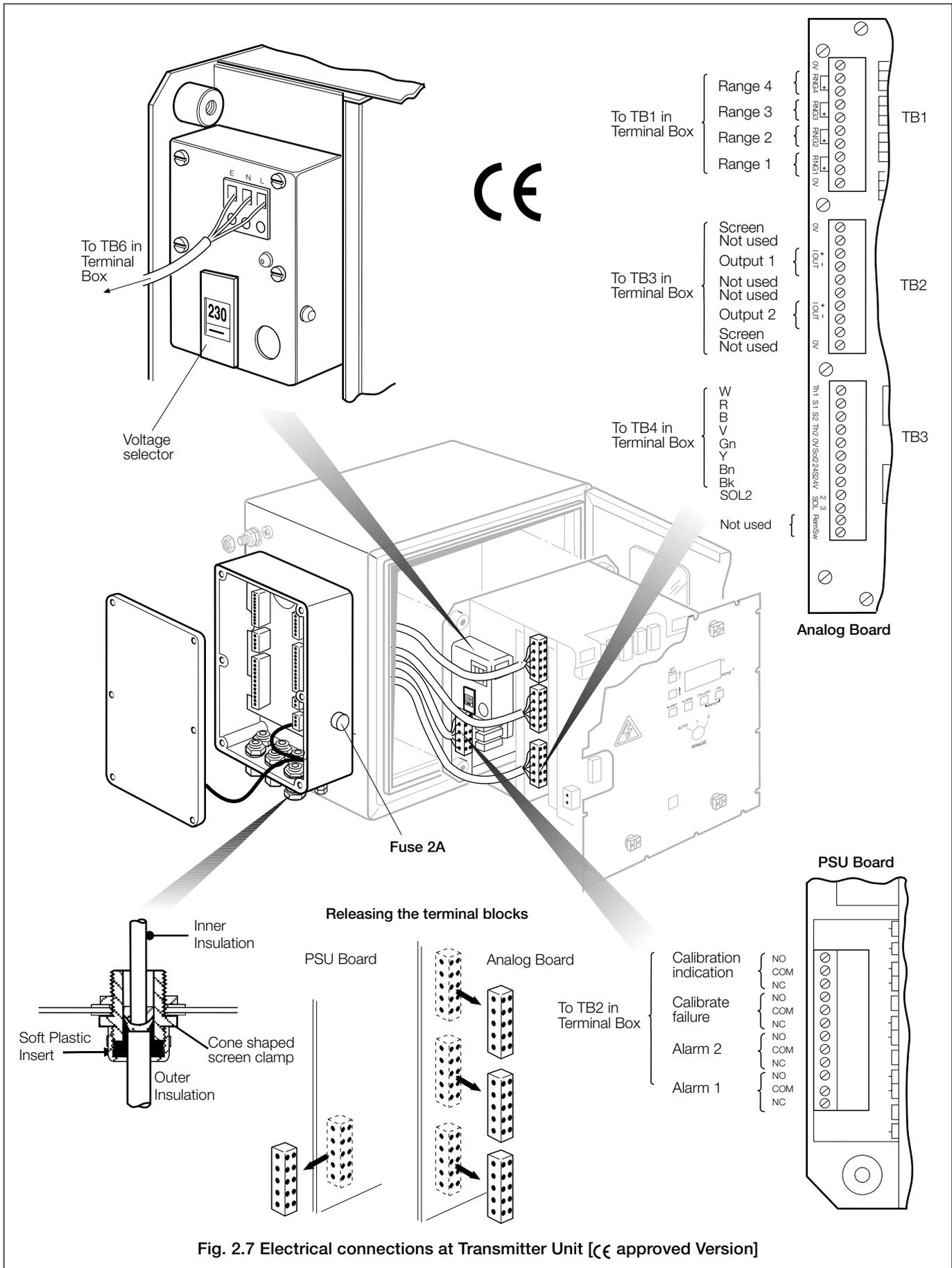
Fig. 2.7 Electrical connections at Transmitter Unit [CE approved Version]
