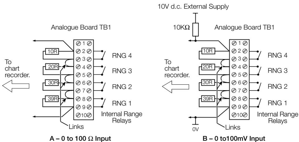
Fig. 2.11 Resistor Network for 'Auto' Remote Range Indication Recorder [Version without CE approval]
