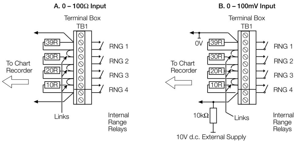
Fig. 2.10 Resistor Network for 'Auto' Remote Range Indication Recorder [CE approved version]
