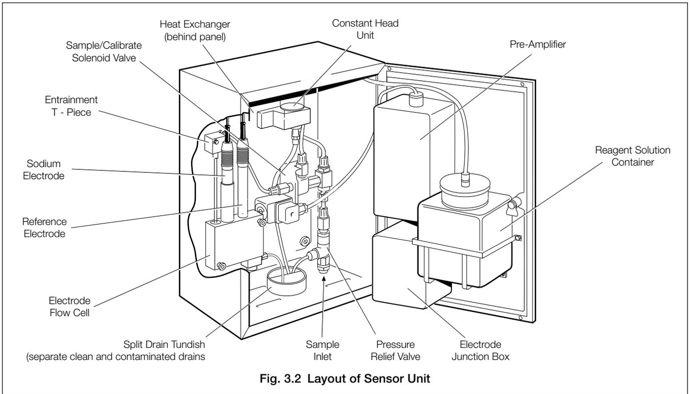
Fig. 3.2 Layout of Sensor Unit
