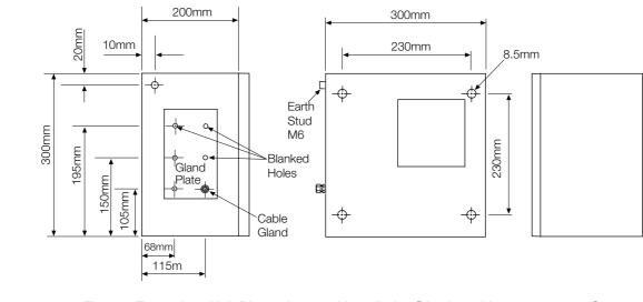
Fig. 2.6 Transmitter Unit Dimensions and Installation [Version without ce approval]
