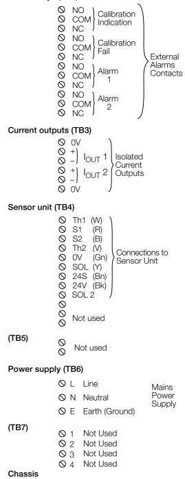
Warning. The power supply earth (ground) must be connected to ensure safety to users, reduction of the effects of RF interference, and correct operation of the power supply interference filter.
