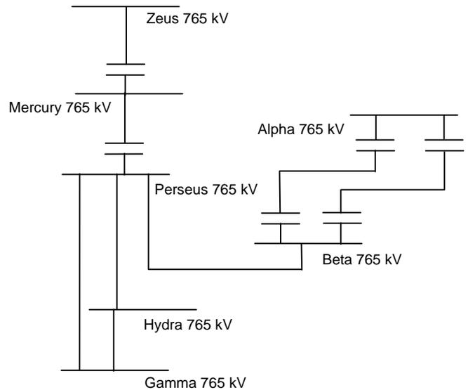
Fig. 1. 765 kV series compensated transmission corridor.
