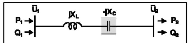
Fig. 2. Series compensated power transmission corridor.
