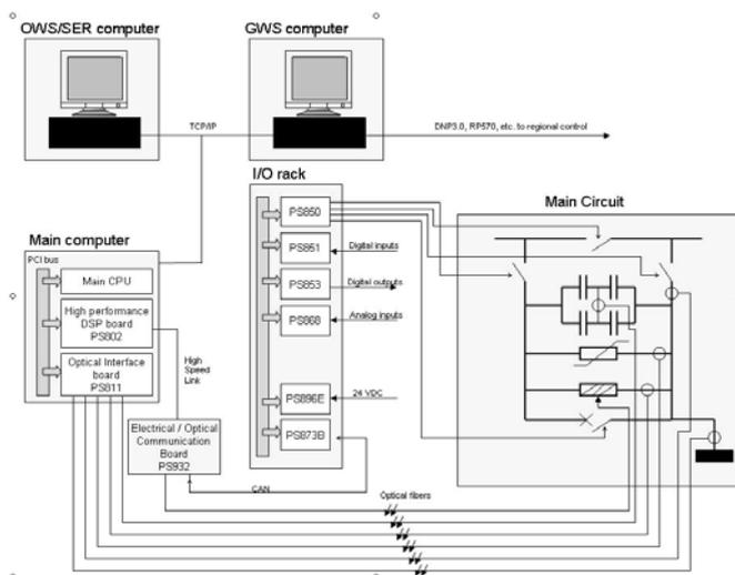
Fig. 11. MACH 2 control and protection system overview.
