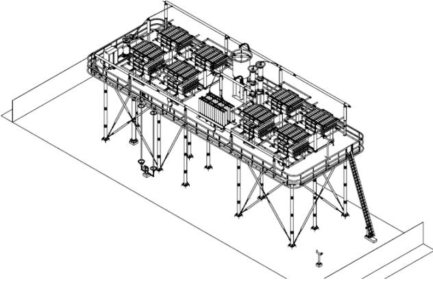
Fig. 12. 765 kV single segment series capacitor lay-out, one phase out of three.
