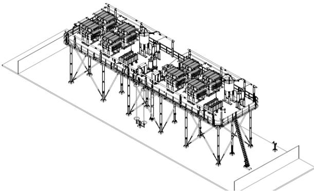
Fig. 14. 765 kV dual segment series capacitor lay-out, one phase out of three.
