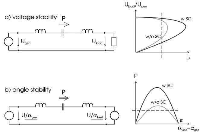
Fig. 3. The impact of series compensation on a) voltage and b) angular stability.
