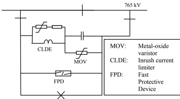
Fig. 7. Single segment series capacitor scheme.
