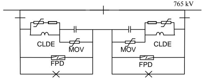
Fig. 8. Dual segment series capacitor scheme.
