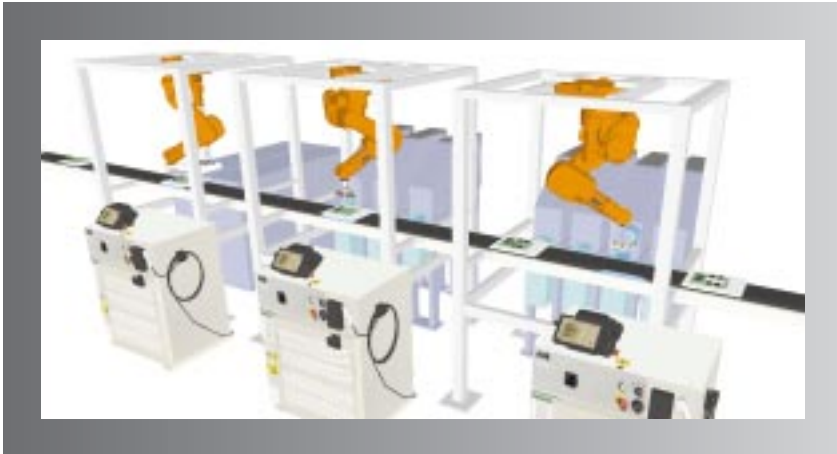
▲ Inverted IRB 140 robots to Clean Room 10 Standards are ideal for assembly and testing of small electronic goods. The robots are compact and are suitable for tight production lines.
