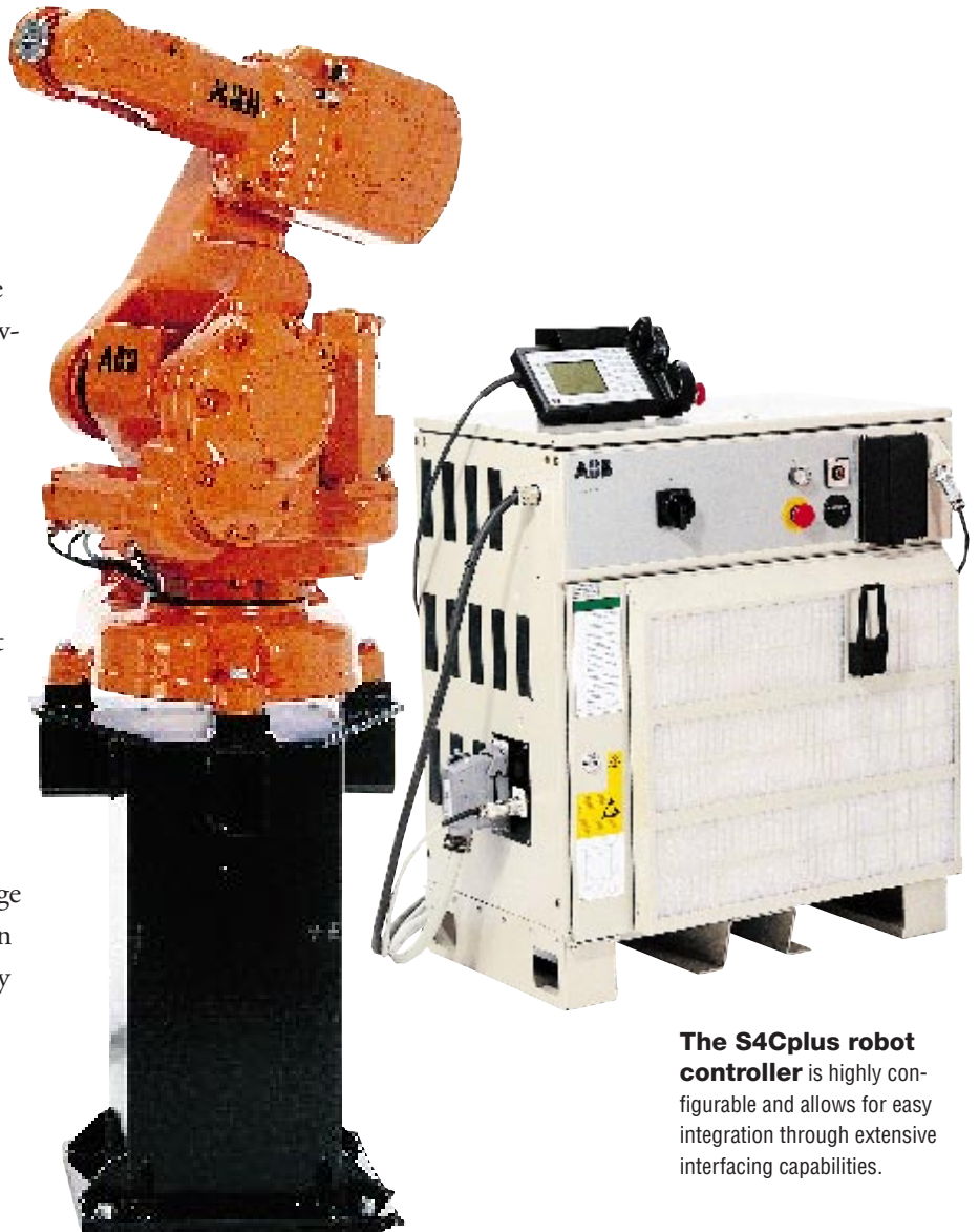
The standard IRB 140 can be mounted at any angle without modification.
