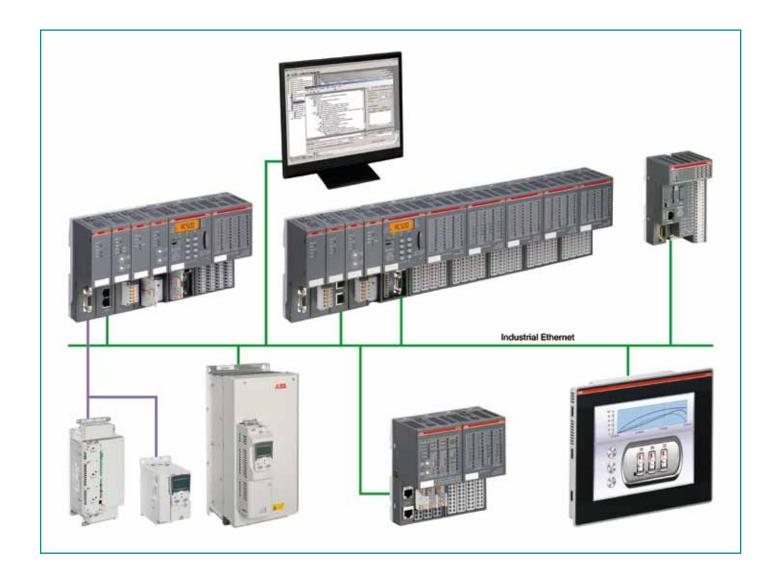
The single-point-of-access is the engineering PC on which PS501 Control Builder Plus is running.
