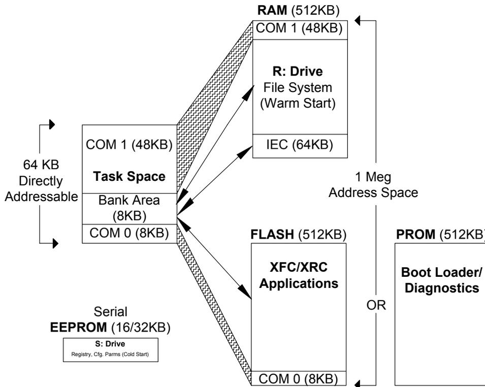
**Figure 2–1 System Architecture for the XSeries XFC and XRC**
