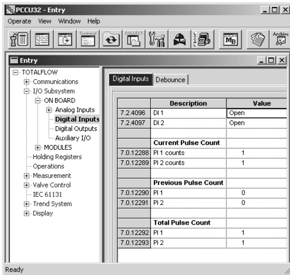
The screenshot shows the PCCU32 - Entry software interface. The left pane displays a tree view of the I/O Subsystem, with 'Digital Inputs' selected. The right pane shows a table of Digital Inputs with columns for Register Address, Description, and Value.
