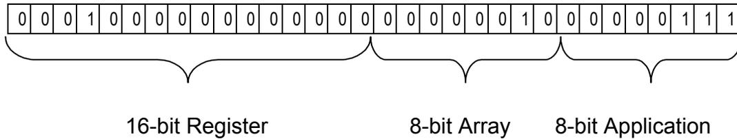
**Figure 4–7 IEC Register ID (32 Bit) Example**
