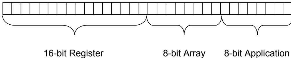
**Figure 2–6 IEC Register ID (32 Bit)**
