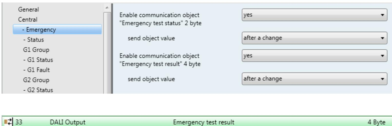
This kind of test result consists of a 4 byte object. Very detailed information concerning the actual converter are included in these 4 bytes. This applies once the latest triggered emergency test mode as well as the detailed test result of the appropriate converter.
