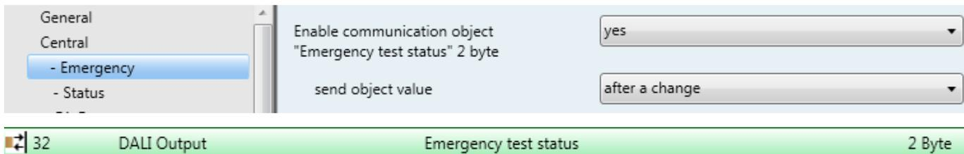
It is also possible to query an emergency light test status. The bit no.7 must be set to 1 in the low byte (address byte).
