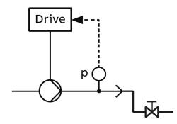
The pressure sensor will not see an increase in pressure during the filling of the pipe in this case, until the pipe is filled.
