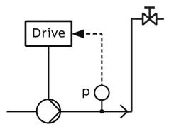
The pressure sensor will see increasing pressure as the pipe is being filled with liquid.
