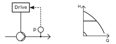
A pressure sensor (p) at the pump outlet is closing the feedback loop for the closed loop control and the PID is controlling the speed based on the provided setpoint
