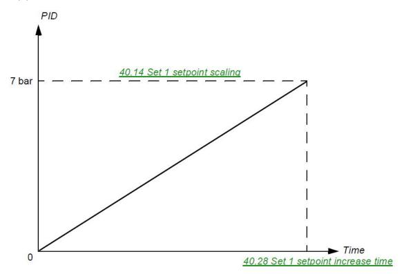
Where the setpoint is gradually increased over time and ending at the full setpoint after the time has elapsed. (The 7 bar is an example)
