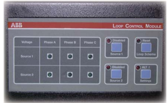
The LCM speeds restoration on distribution power systems.
