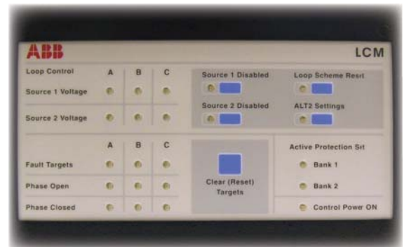
The enhanced LCM adds individual phase targets, recloser position, and displays both banks of protection groups.
