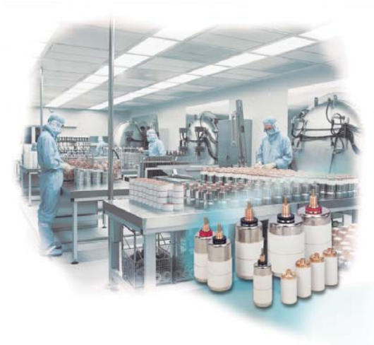
ABB vacuum interrupter clean room
