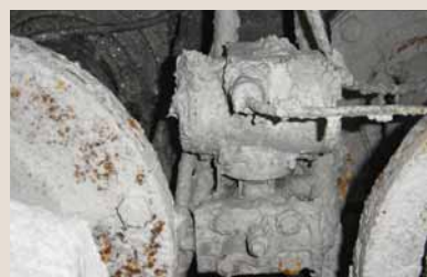
1 Temperature sensors and a TTH300 transmitter
