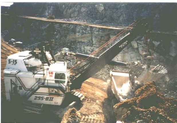
Figure 1: First shovel with ABB LV AC Drives in Mexico, 1999
