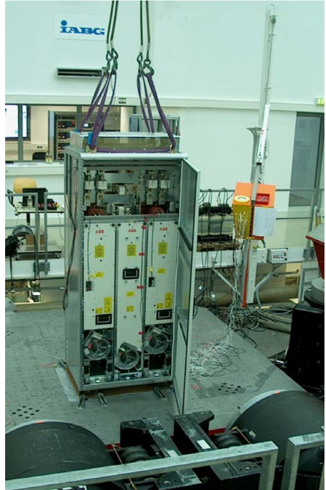
Figure 5: Shaking table and test unit, Munich, 2005
