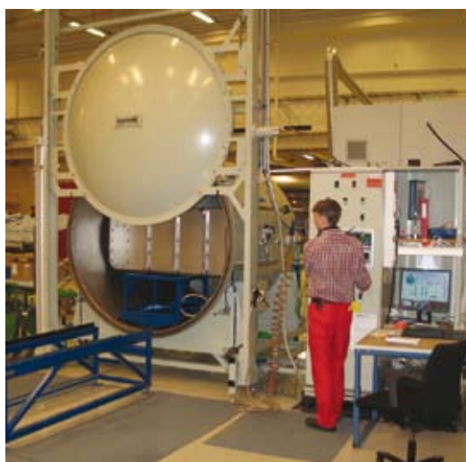
Vacuum chamber for leakage test and \text{SF}_6 gas filling
