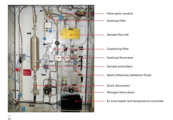
01 Sample conditioning system including fast-loop, flow cell and automatic wash.
