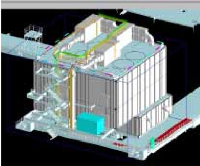
**Figure 6: Sketch of two 40 MW VSC HVDC offshore module excluding the motor located on the platform deck.**
