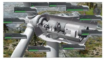
For the 3-D design, a connection between the application, which resides on a mobile device or desktop PC, and the database containing the plant data was implemented. This real-time connection allows field personnel to instantaneously obtain information about the asset while they are performing repair and maintenance work.
