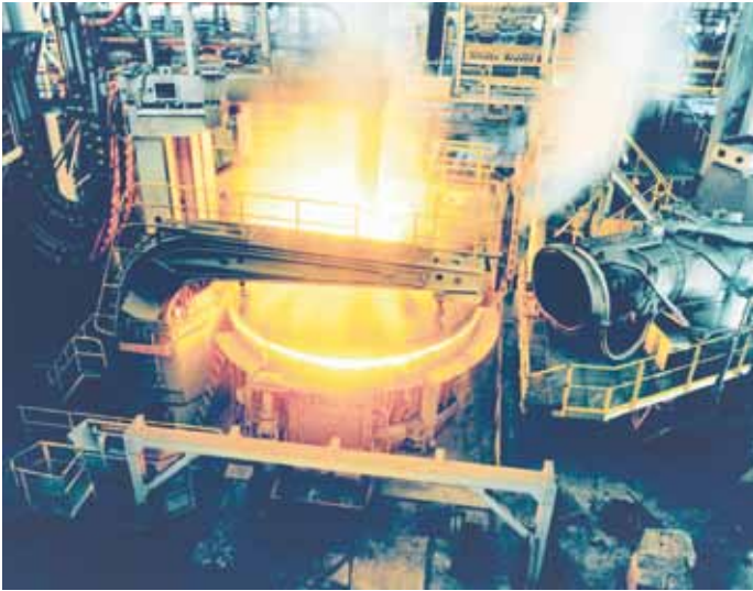
Electric arc furnace.
