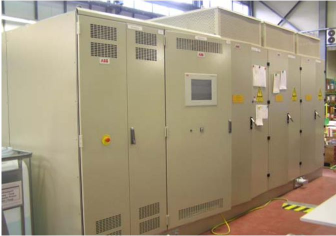
Figure 5. Cycloconverter with new controller generation during testing in the factory.
