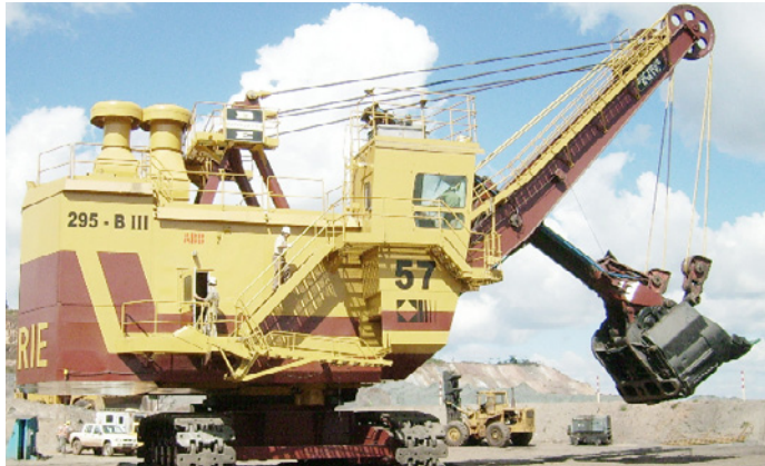
A Bucyrus-Eerie model 295-B III electric shovel from Itabira – Vale Brazil, retrofitted with modern ABB AC drives and control system.
