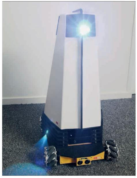
In order to augment the reality with the overlaid annotation from the expert, the robot uses a compact projector embedded in its body.
