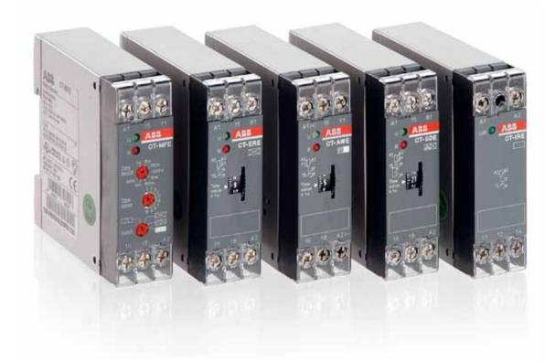
The CT-E range with its excellent price/performance ratio offers an ideal solution for serial applications. 56 single-function devices with 5 different time ranges as well as 2 multifunction timers with 6 functions and 8 time ranges offer the highest possible flexibility for almost every application. For high operating cycles, contact-free CT-E timers with solid-state output are available.
