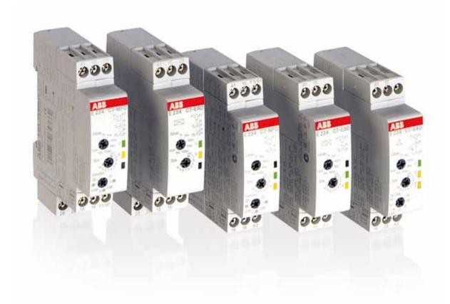
The CT-D range represents a link between industry and the installation types. For maximum flexibility in operation, 10 single-function as well as 2 multifunction devices with 7 timing functions are available. The devices offer 4 or 7 time ranges from 0.05 seconds up to 100 hours. Their wide input range allows use in applications worldwide.
