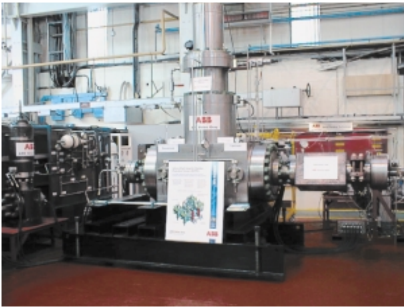
High Integrity Pipeline Protection System (HIPPS) under test in the laboratory
