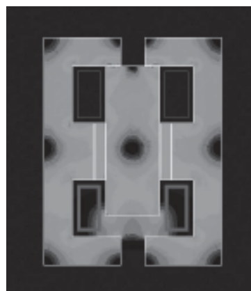
Fig. B Magnetic circuit with opening coil supplied.
