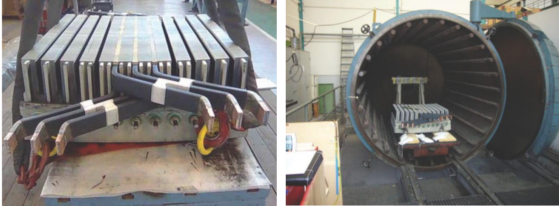
Figure 12 – Insulation tests in hypobaric chamber simulated at 5,000 masl
