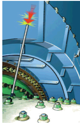
Figure 11– Challenge to access the last row of liner bolts
