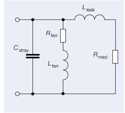
**Simplified schematic of the equivalent circuit diagram in Fig. 3** **4**
