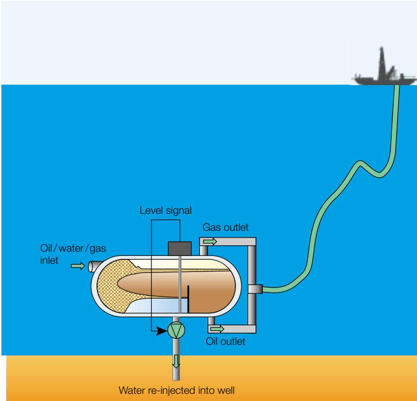
**Subsea separation and injection system (SUBSIS). Level signals from the new inductive level monitoring system are used to control the water pump. (In the Troll Pilot project the gas exits through the oil outlet.)** 1
