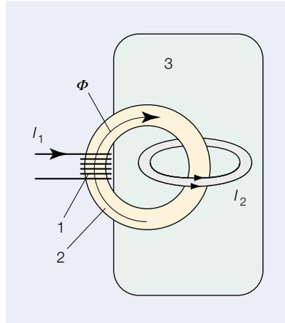
**Inductive principle and possible arrangement for detecting the conductivity of a surrounding medium** [2]
