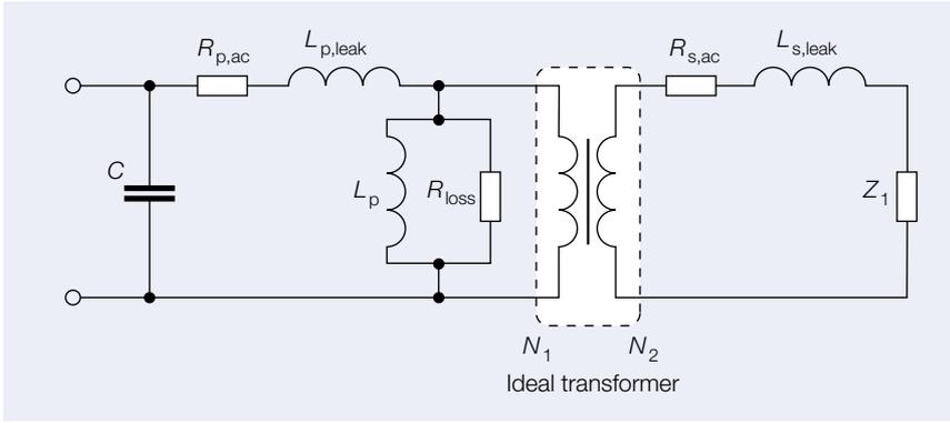
**Equivalent circuit diagram of the 'transformer' used to explain the inductive sensor principle** **3**
