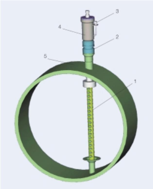
**ILMS developed for use in subsea separators**
