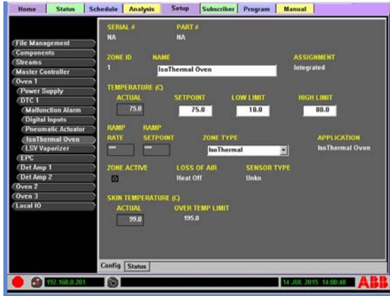
Fig. 6.41. Isothermal Oven Configuration Example
