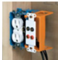
Attaching the add-on bracket is a “snap.” Just remove the back of the double-sided tape (1), clip the bracket in place (2) and press on the bracket to secure it against the box (3). Enables the installation of most rectangular yoke plates.
