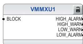
Figure 139: Voltage measurement: Three-phase voltage measurement (HV side)
