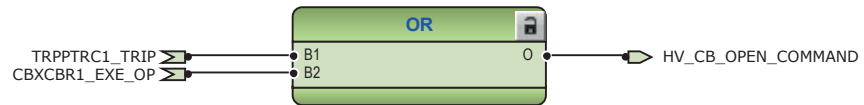
Figure 39: Circuit breaker control logic: Signals for opening coil of high-voltage side circuit breaker
