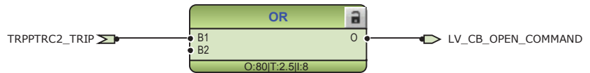
Figure 83: Circuit breaker control logic: Signals for opening coil of low-voltage side circuit breaker
