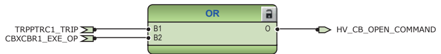
Figure 129: Circuit breaker control logic: Signals for opening coil of high-voltage side circuit breaker
