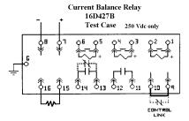
Contact 13-14 convertible External resistor supplied with relay
