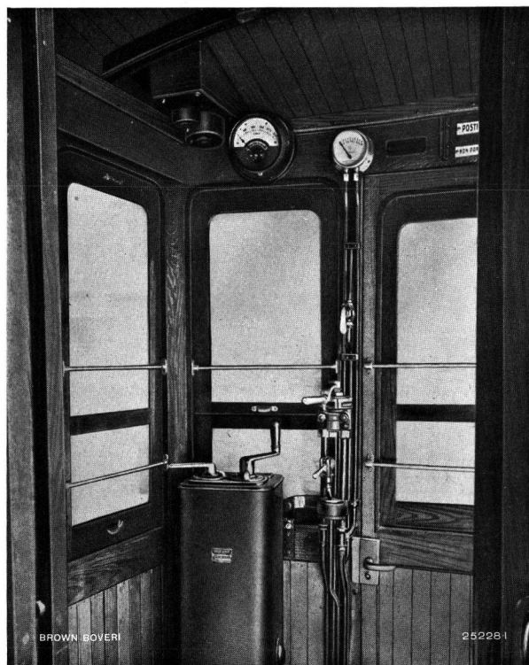
Fig. 3. — Driver's cab with master controller and reversing drum combined.
