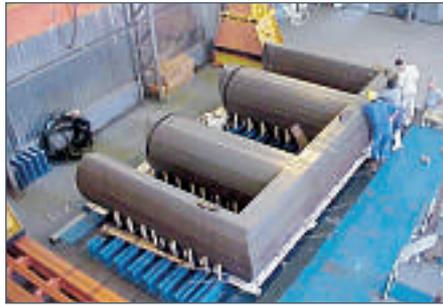
All parts delivered from the factory, such as windings and main insulation, had already undergone intensive in-factory tests. Measurements such as winding ohmic resistance, voltage ratio (with auxiliary test core), measurements of leakage magnetic flux and applied voltage between parallel conductors had been recorded.
