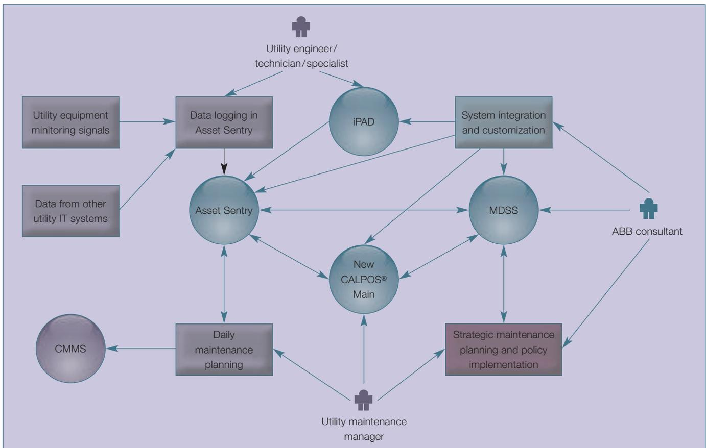
performed in the MDSS web HMI, the utility maintenance manager has options to review the rules that triggered the resulting condition and to request further analysis of the condition by 'asking' an ABB expert **7**.
