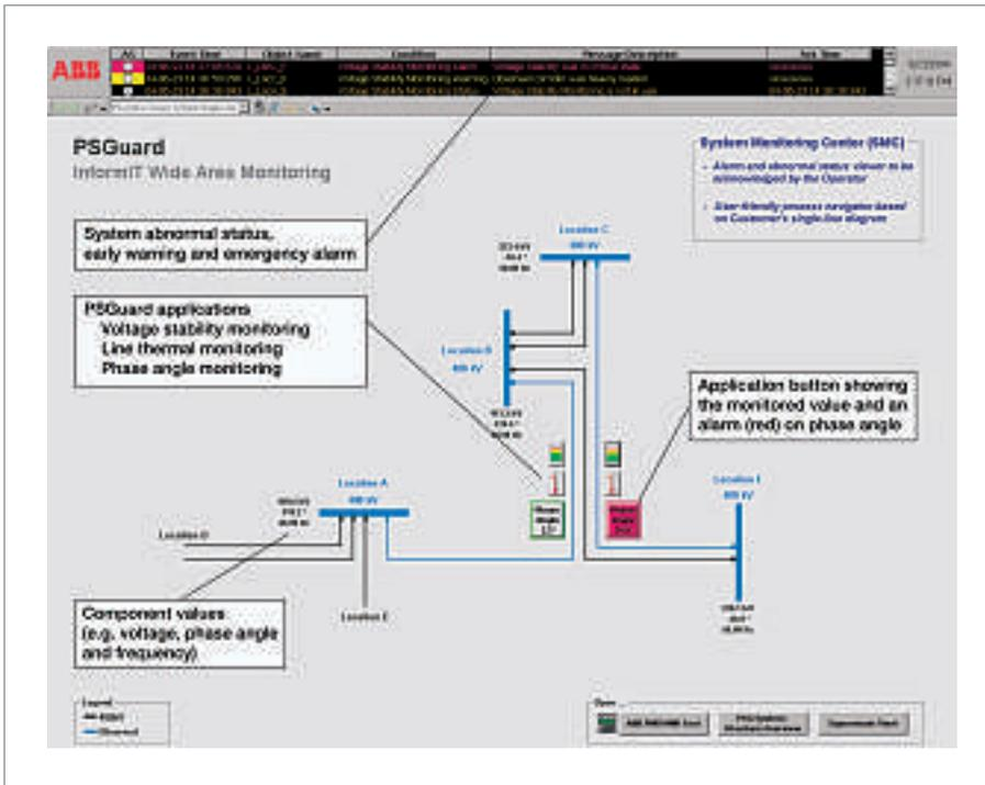
and the voltage phase angle difference is observed. An active power transfer via two monitored lines and its relation to the voltage phase angle difference
