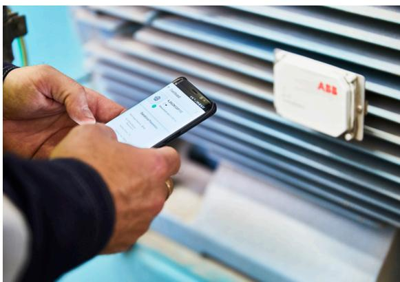
**Smart sensors monitor key parameters to provide detailed insights into the performance and health of motors. As a result, maintenance can become predictive rather than reactive.**
