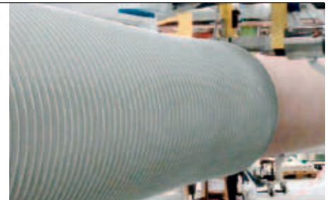
6b Seamless extruded silicone housing
