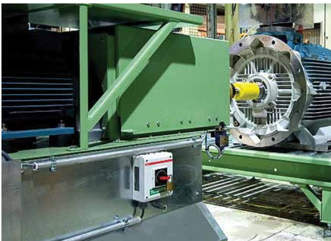
Safety switches can be padlocked in OFF position
