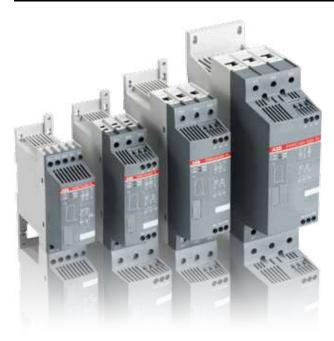
PSRC is a unique softstarter designed specifically for scroll compressors, that is very easy to use and install. The PSRC softstarter was designed with a short starting time whilst maintaining a low starting current thus increasing the life span of the compressor. As the settings cannot be changed, reliability is guaranteed.
