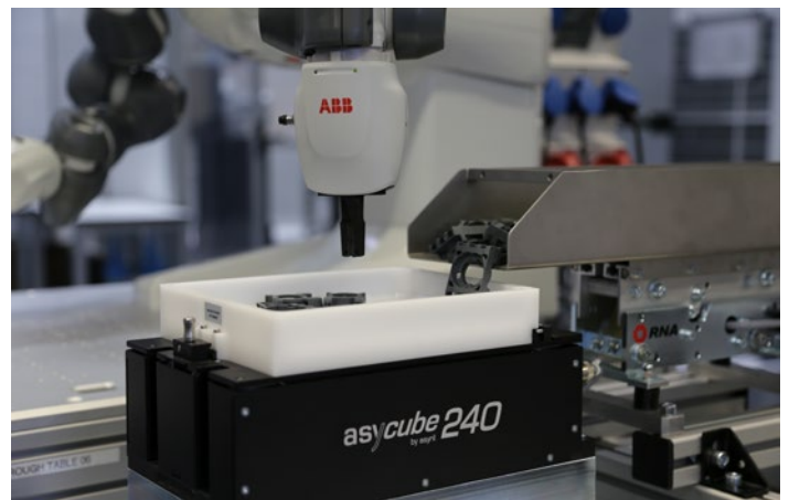
The part hopper is available in different sizes (image shows 2 L version)
