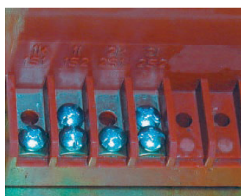
Fig. 2. 2 Secondary terminal box (2 secondaries and grounding screw)
