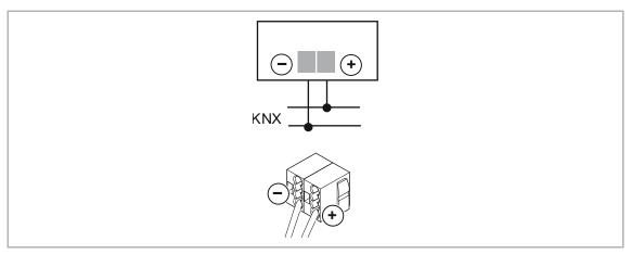
Fig. 12: Electrical connection
