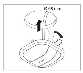
Carefully slide the connected device into the recess.
