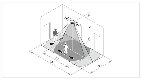
Fig. 16: Detection ranges of Busch-Presence detector Corridor KNX / Busch-Presence detector Corridor Premium KNX [H] Mounting height
