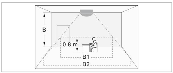
Fig. 14: Detection ranges of Busch-Presence detector KNX / Busch-Presence detector Premium KNX
