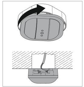
Now turn the device in a clock-wise direction until it is aligned with the surface-mounted housing.
