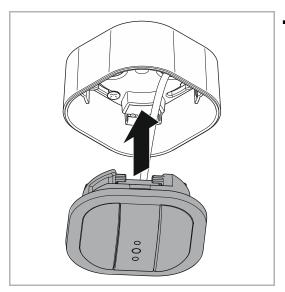
Now slide the connected device into the surface mounted housing according to the illustration shown opposite. Take note of the guide rails. This is the only way the device can be inserted!
