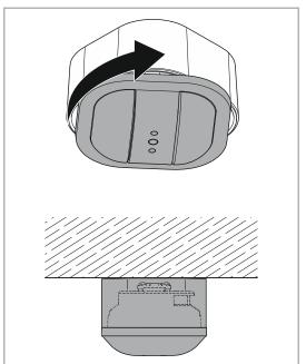
Now turn the device in a clock-wise direction until it is aligned with the surface-mounted housing.
