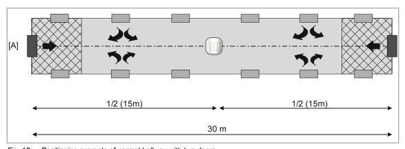
Fig. 18: Positioning example of normal hallway with two doors
