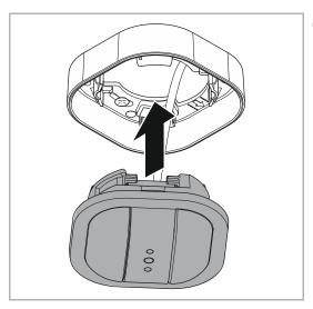
Now slide the connected device into the intermediate ring according to the illustration shown opposite. Take note of the guide rails. This is the only way the device can be inserted!
