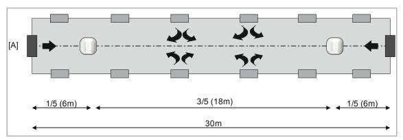
Fig. 19: Positioning example of normal floor smoke section with 2 doors
