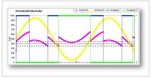
Fig. 22: Time sequence of the constant light switch.
