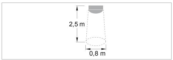
Fig. 20: Detection range of the sensor for brightness detection (does not apply to the Busch-Watchdog Sky KNX).
