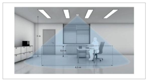
Fig. 5: Inner detection range
