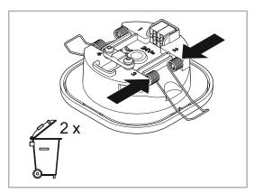
Remove the two clamps on the device with the aid of a screwdriver and dispose of them.
