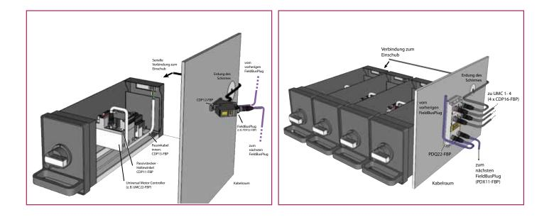
The UMC100-FBP is ideally suited for plug-in applications in Motor Control Centers. Here, the UMC100-FBP is positioned within the slot while the FieldBusPlug fieldbus connection is mounted externally. Communication is undertaken by means of a simple serial link.
