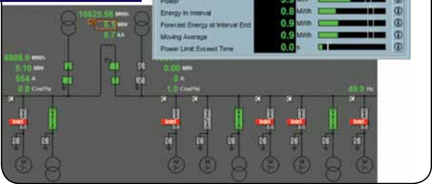
Figure 9: integrated electrical energy monitoring and management
